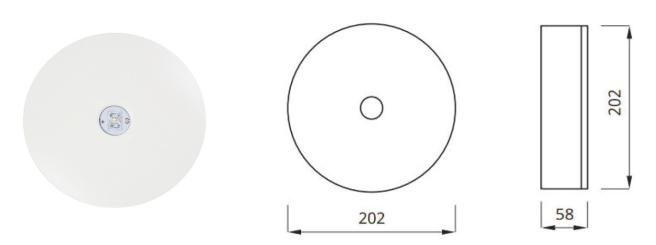
A stylish and compact circular IP65 3 Watt or 6 Watt LED Bulkhead suitable for ceiling mounting applications. Offered as either 390 lumens (3W) or 600 lumens (6W) this is an excellent solution for tall ceiling heights in damp locations. The unit utilises LiFePO4 battery technology which provides a far longer life than traditional battery types, making this an ideal product for difficult to maintain areas.
