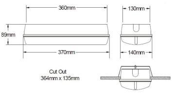
The EDW is a high output emergency LED bulkhead which is designed for high ceiling applications. The high output LED strip use in this fitting provides 444 & 395 lumens after the diffuser in both mains and emergency operation respectively.
