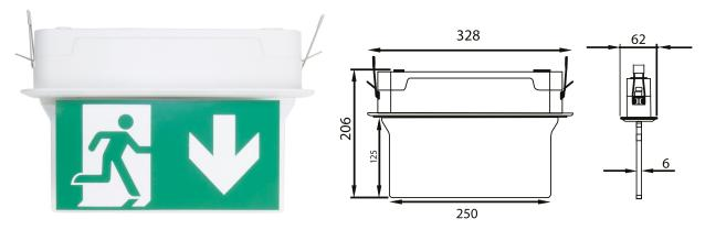
A stylish and compact Double Sided LED Exit Sign suitable for ceiling recess mount applications. The unit is available in either a Switchable Maintained/Non-Maintained or DALI Self-Test version.
