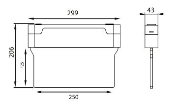
A stylish and compact Double Sided LED Exit Sign suitable for ceiling surface mount applications. The unit is available in either a Switchable Maintained/ Non-Maintained or DALI Self-Test version.
